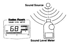
The meter begins to display the *continuous* average sound level. This is the average sound level during a 1-second sampling period, which the meter updates once per second. The bargraph shows the continuous average for either a 0.2-second or 0.5-second period, depending on the response setting.
