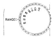
Set RANGE for the approximate sound level you want to measure. If you do not know the sound level, start with the highest range setting (120) and gradually reduce the setting. When the measured value is lower or higher than the set range, an under range or over range indicator appears. See "Level Indications."
